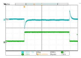
Figure 12. Load Transient VOUT=5V, IOUT=0.2A to 1.8A, SR=250mA/us
