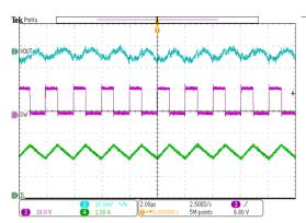
Figure 10. SW node waveform and Output Ripple, IOUT=2A
