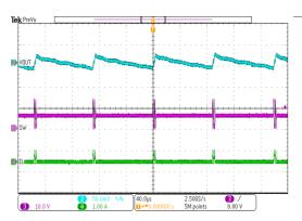
Figure 11. SW node Waveform and Output Ripple, IOUT=10mA
