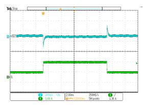
Figure 13. Load Transient VOUT=5V, IOUT=0.5A to 1.5A, SR=250mA/us
