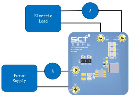
Figure 1. Proper Supply, Load and Measurement Equipment Setup
