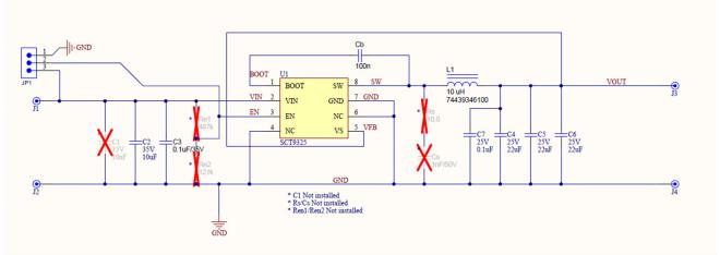
Figure 3. SCT9325 Evaluation Board Schematic
